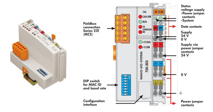
This buscoupler allows connection of the WAGO→I/O→SYSTEM as a slave to the CAL fieldbus. The module data is transmitted using Communication Objects (COB).
