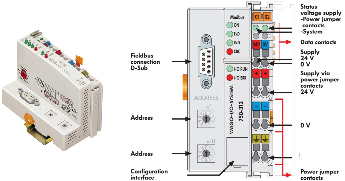
This buscoupler allows connection of the WAGO I/O SYSTEM as a slave to the MODBUS fieldbus.
